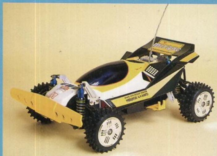
1/10 MIRAGE 4WD OFF-ROAD BUGGY 1553 RS-540S powered with shaft-coupled twin differentials, sliding-spline drive shafts, double wishbone independent suspension and oil-filled shock absorbers.
